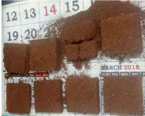
Fig VII: Direct Shear test
