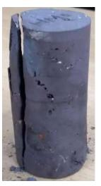
Figure V. Determining UCS of rock sample
