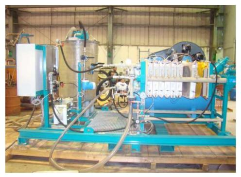
Fig. 3.8 Pilot scale pressure filter set up
