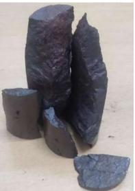
Fig VI: Triaxial Setup and Fractured Sample
